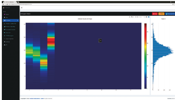
Position heatmap (counts over position) corresponding to four different ^3\text{He} tubes and 2D-projection of counts onto the y-axis of a single tube.
