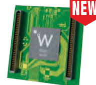
PSIROC Psiroc is a 64-channel front-end ASIC designed to readout PIN diodes, silicon strips and GEMs, handling detector capacitances ranging from 0 up to few hundreds of pF.
