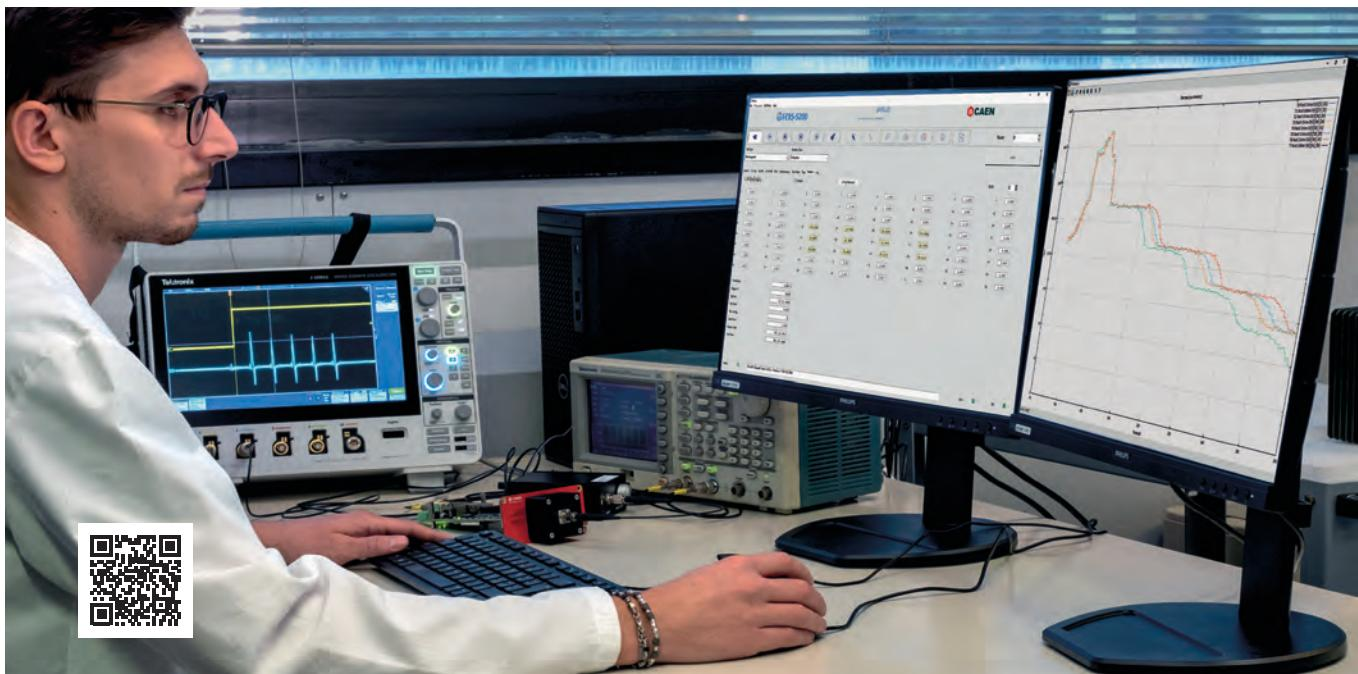
**A single DAQ software to control the FERS-5200 board family. Available in Console and GUI Mode, it allows the user to customize the DAQ, and offers an easy way to approach multi-boards and high-channel density FERS-5200 systems.**
