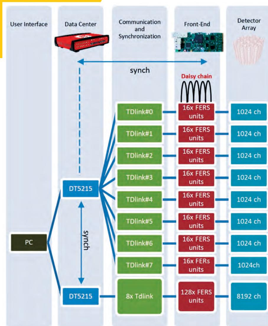
The DT5215 Concentrator Board is responsible for synchronization and data collection from multiple FERS units. It features 8 optical TDLink connectors, each with the possibility of controlling up to 16 FERS units in daisy-chain, for a total of 128 cards per concentrator. Multiple concentrator boards can be synchronized in order to further extend the total number of channels.
