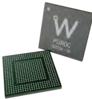
Charge measurement is done with peak detectors but those can be used in a track & hold fashion thanks to an internal delay cell. Analog data are outputted on two multiplexed analog output and can be read-out with an external ADC. Shapers shaping time can be adjusted from 20 ns to 3  $\mu$ s with a step of 20 ns up to 300 ns and a step of 200 ns up to 3  $\mu$ s. Data acquisition can be done ASIC wide or channel-wise.
