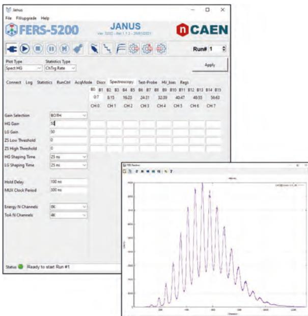
Janus is composed of two parts, one written in C, which is the real heart of the application, one written in Python which manages the user interface. The plots are executed through Gnuplot. All the configuration parameters are written in a textual configuration file.
