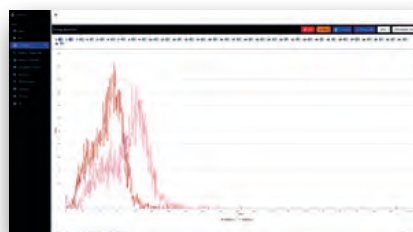
Energy spectrum measured at the two ends of one ^3\text{He} tube – x-axis is not-calibrated energy.
