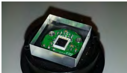
Scintillating tile coupled to a sensor.
