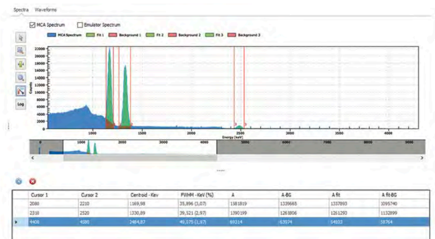
The ^{60}\text{Co} complete spectrum acquired by the MCA DT5770 and plotted by the Emulation Software
