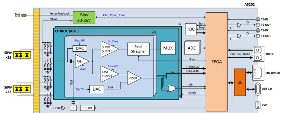
The A5202 can be controlled as a standalone unit via USB or Ethernet using **Janus readout software**.
