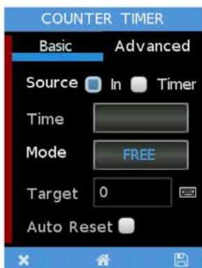
Each function can be programmed using the widget on the touchscreen
