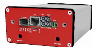
DT5215 Concentrator Board (left) and A5202 boxed for desktop use (right)
