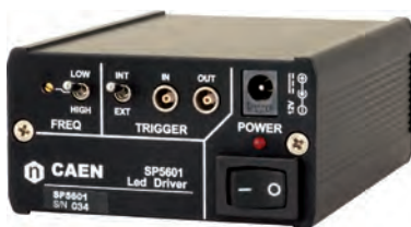
The SP5601 is an ultra-fast LED Driver with pulse width at ns level, tunable intensity and frequency, that provides a low-cost tool for the detector characterization. The LED pulse generation can be triggered by an internal oscillator or by an external pulser.
