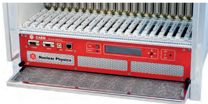
VME8200 is provided with a 1U, removable air filter to safely cool down the VME modules operating within the crate.
