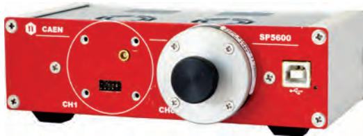
The SP5600 is a general purpose Power Supply and Amplification Unit, integrating up to two SiPMs in a mother & daughter architecture allowing for easy mounting and replacement of the sensors. Each channel can provide a digital output generated by the fast leading edge discriminators. A timing coincidence of the two channels is also available.
