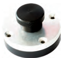
The SP5650C is a sensor holder provided in the Educational Photon kit. The holder hosts a 1.3x1.3 mm 2 Silicon Photo- Multipliers; moreover, a probe inside the holders senses temperature variations, thus allowing the user to compensate for possible gain instability. The SP5650C is made of a mechanical structure providing a FC fiber connector and a PCB where the SiPM is soldered.
