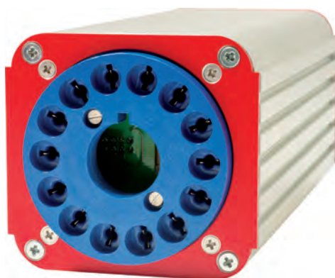
γstream rear view. Internal divider can be adapted for NaI(Tl), LaBr 3 (Ce), CeBr 3 detectors with standard 14-pin and 10-8 stages PMTs.
