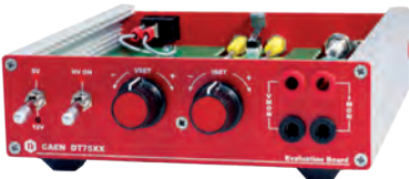
A desktop evaluation board (Mod. DT75xx) is available for easy testing of the A750x modules.
