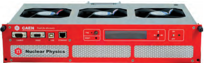
The 2U Smart Fan Unit shows a 4-directional switch, OLED display and various interfaces (CAN bus, Ethernet, USB, RS232) for local and remote control of the crate. The user can easily monitor all the operational parameters as supply voltages, fan speed and temperature.
