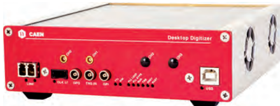
The DT5720 is a CAEN Desktop Waveform digitizer housing 2 channels 12 bit 250 MS/s ADC with a dedicated charge integration firmware for real time pulse processing.
